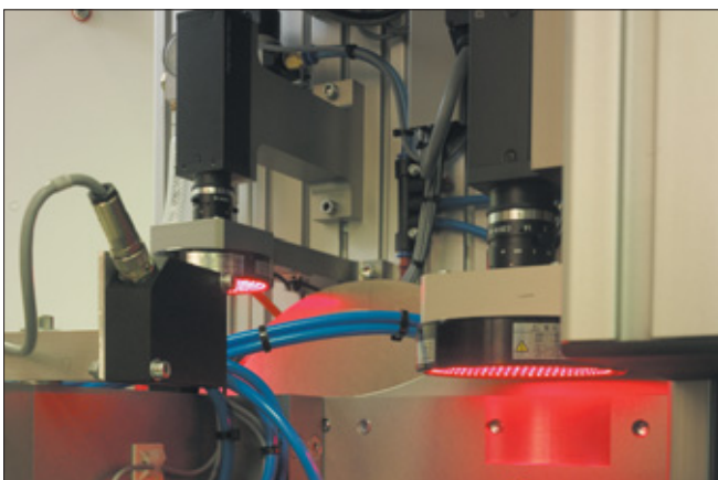
1 x laser micrometer, 3 x image processing cameras
